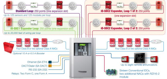
Each iO1000 panel has room for up to two Signature loop controller modules in any combination of single or dual 250-device loops. iO1000 loops support 125 detectors and 125 modules.
