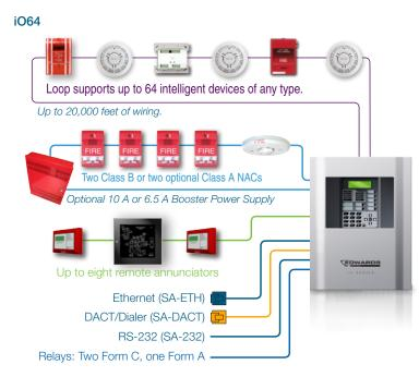
Each iO64 panel ships with one Signature loop controller that supports 64 devices of any type. This panel's device capacity cannot be expanded.
